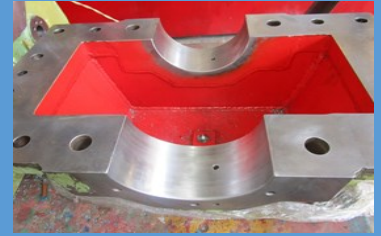
As-repaired Bearing Pedestal
