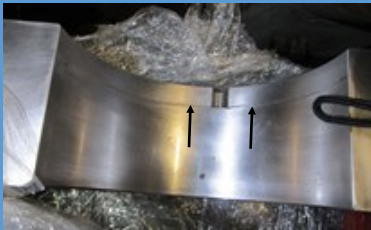
Crack along Bearing Pedestal
