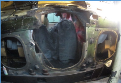
Damaged Engine Crankcase Window
